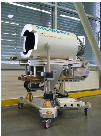
Figure 10: setup for an easy to exchange head gradient insert allowing higher performance
