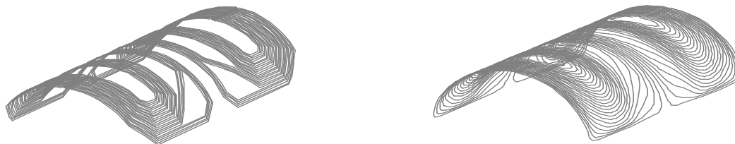
Figure 8: Gradient coil winding design of a transverse gradient coil (Y). Left: Polygon design. Right: Finger-print design.
